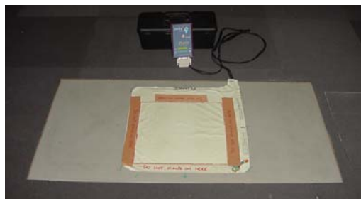
Figure 4.2.2: Photograph of the pliance® pressure mat placed over the top of the AMTI force plate.
