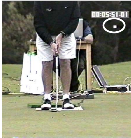
Figure 5.2.1.2: Image capture from video indicating the Peak synchronization event used to synchronise the pliance® and video systems.
