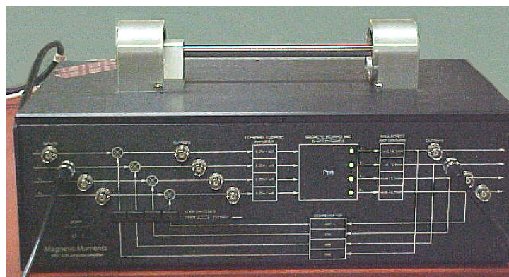
Figure 4.21 MBC 500 magnetic bearing levitated using the designed digital controller on channel 2
